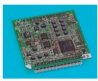
DS-SS Modulation/ Demodulation Engine for PLC
