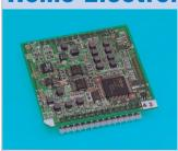
demodulation engine for PLC
