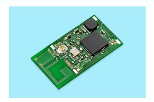
SMK Corporation has developed a miniature thread-compliant low power RF module with built-in antenna.
