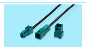
SMK Corporation has developed automotive small coaxial connectors "MH-2 Series". With the commonized housing, it allows the connection of cables of two different thicknesses; 1.5D and 2.5D. Board plugs for connecting coaxial cables to boards are also available.
