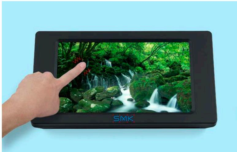
SMK Corporation has developed One Glass Solution (OGS) capacitive touch panel with Force Feedback (FFB) “CapBeat Touch OGS”. The FFB touch panel uses SMK’s unique technology to make touch panel vibrate by piezoelectric elements.
