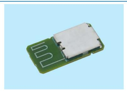
SMK has developed a small Bluetooth<sup>®</sup> low energy module "BTS05 series" supporting Bluetooth<sup>®</sup> Version 5.0. It is compliant with 2M PHY for LE, the physical layer specification which is added as part of Bluetooth<sup>®</sup> Version 5.0, contributing to an improved transmission speed compared to the SMK's previous product.
